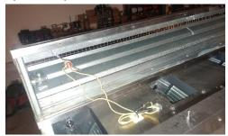
Locate the electric connectors, and while grasping the connector itself (not the wire), unplug unit
